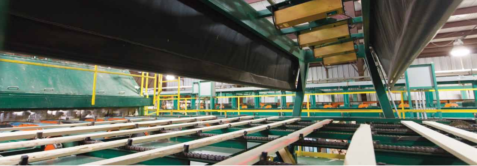
JoeScan scan heads provide information on the sides of the board and identify wane.
