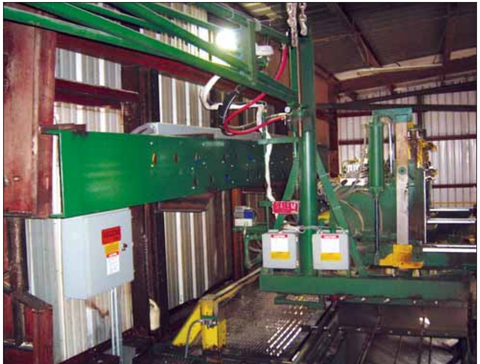
JoeScan scanners behind the carriage capture data from the back of the log (pictured).
