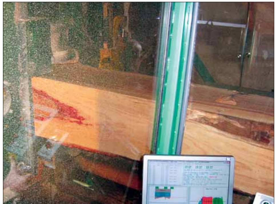
Sawing a red oak log at Al-Tom Forest Products on new Salem carriage; head saw is a Salem 6-foot airstream bandmill. The head rig was optimized with JoeScan scanners and Nelson Brothers Engineering optimization system.
