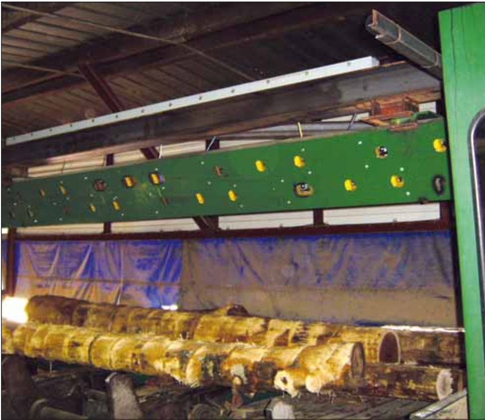
JoeScan scanners above the log deck infeed capture data from the front of the log.
