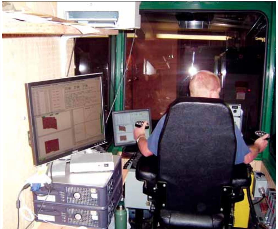
View of the interior of the sawyer's cab with computerized controls. 'It's a lot easier to train a sawyer now that we have the Nelson Brothers optimization equipment in place,' says operations manager Coby Crager. 'It takes a lot of the decisions off the sawyers.'
